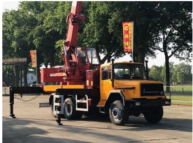
Iveco 256-26 AK 6x6 - Crane HMK420T
